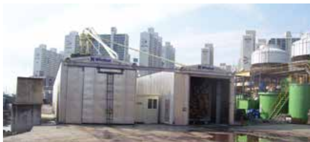
Windsor log conditioning chambers offer a simple effective system for softening logs.
